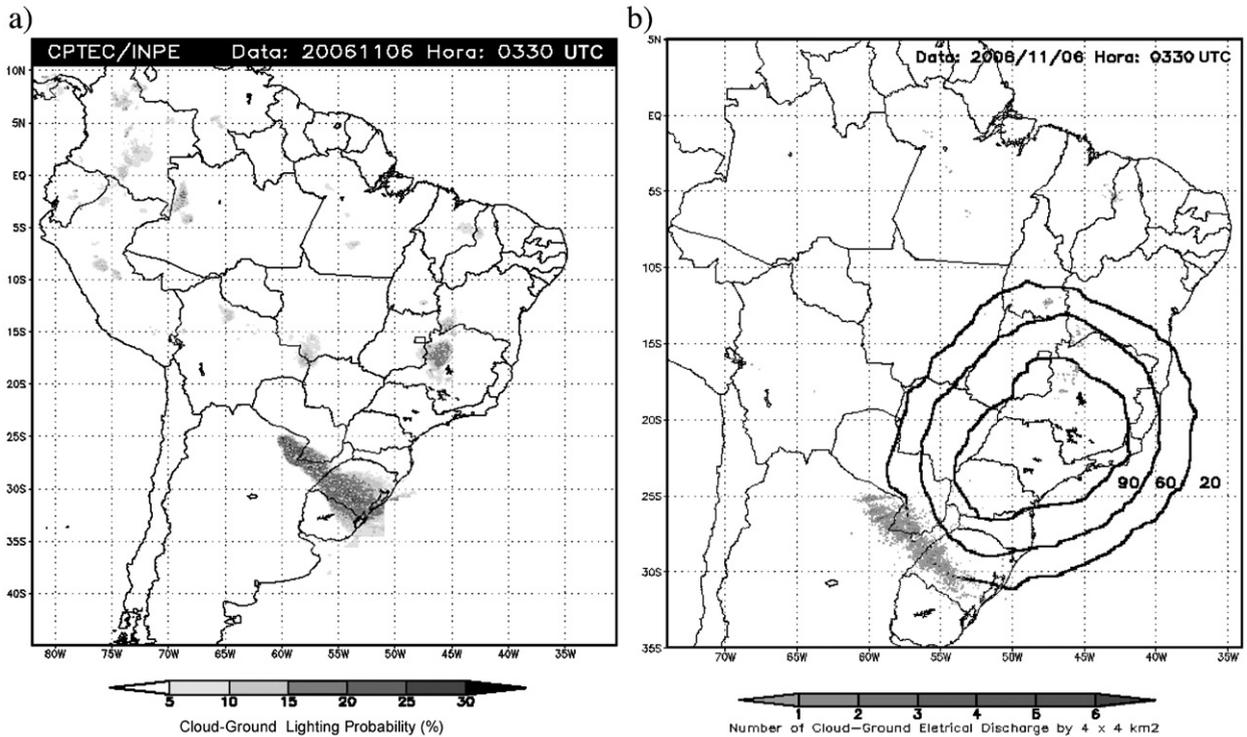
**Fig. 5.** a) Probability of lightning occurrence for November 6th 2006 at 03:30 GMT. b) Number of cloud-to-ground discharges per pixel 7.5 min before and after 03:30 GMT on the same day.
